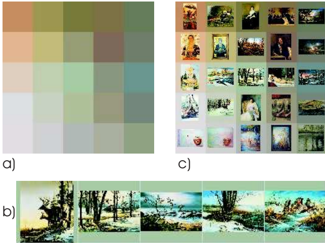
Figure 4: a) A 5 \times 5 SOM visualising a set of bitmap images characterised by colour-histogram vectors. Each square is coloured in the mean colour of the codebook vector's histogram. b) Thumbnails of the images quantified by a selected node, in this case the centre node. Each node in the map quantifies a small easily-browsable number of similar images. c) Thumbnails of closest images may be used to describe the codebook vectors.
