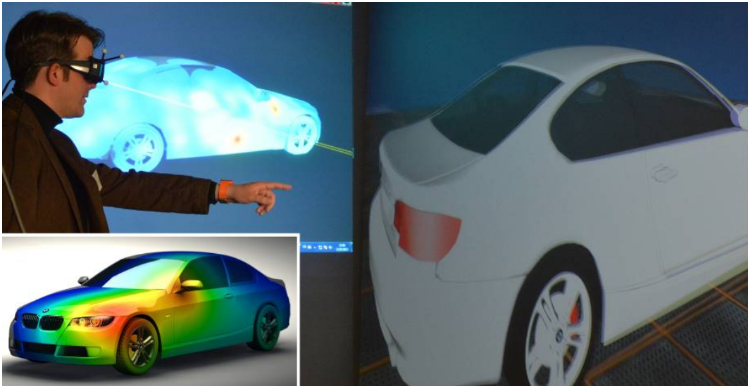
Figure 1: The presented approach is able to map fixations to 3D models of the environment and create 3D heatmaps in real-time. The example shows a 3D gaze recording in an immersive virtual environment (person to the left inspecting 3D object on the right). Real-time heatmap generation is shown in the left background (wrong colors due to photography of a projection screen). Lower left corner shows a rendering of the created 3D heatmaps.
