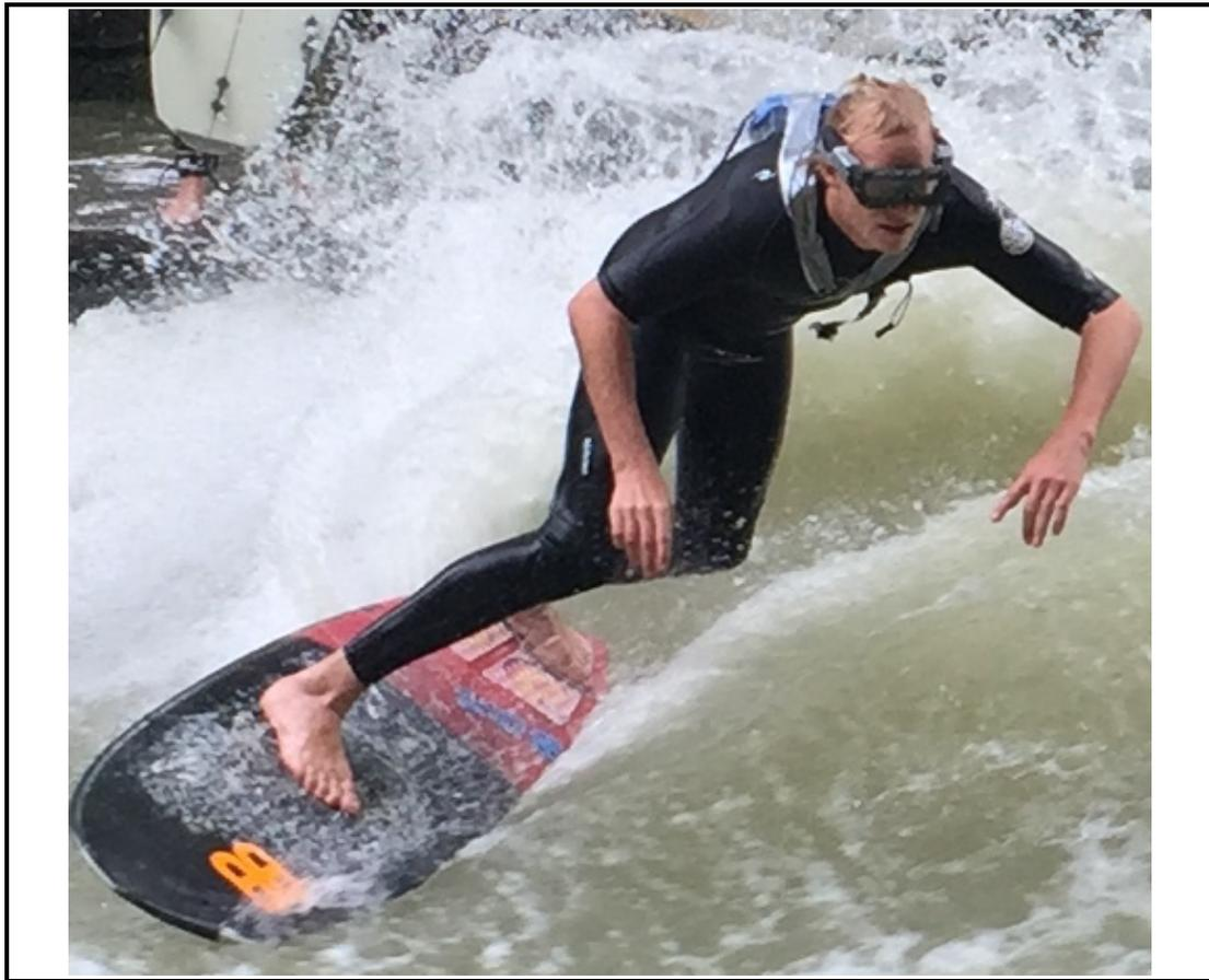
Fig. 1. An expert surfer performs a carve turn whilst wearing the *Tobii Glasses 2* in the water-housing system and the recording-unit on his back.
