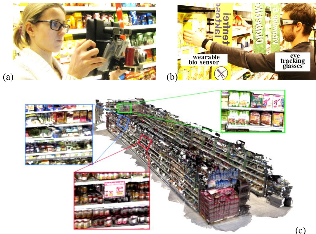
Figure 1. Hardware (a) for the 3D model building process (Kinect and HD camera), (b) study with packages, (c) 3D environment model, a large shop floor.
