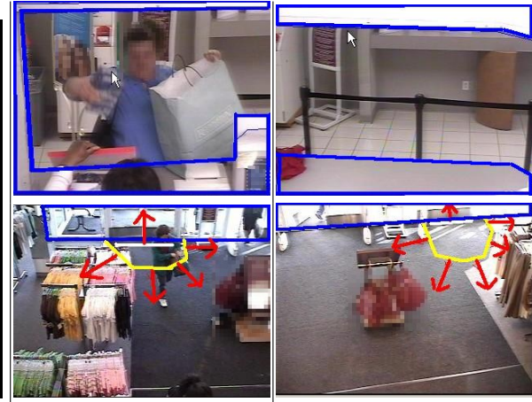
Fig. 2. Views from four of the six cameras — two at the customer service desk (top) and two of the four doors (bottom). The “region of uninterest” is shown in blue for all frames and the entrance tripwires ( enter in yellow, leave in white) are drawn on the views.
