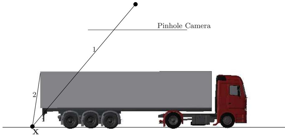
**Fig. 4.** The bird's-eye view system. First, pixels of the resulting virtual image are projected onto the ground plane and then they are projected to omnidirectional images where the pixel values are constructed by bilinear interpolation.
