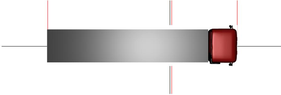
**Fig. 5.** Several subdivisions to construct bird's-eye view images. The black lines show the division into the cells of points closer to each camera than to any other camera with the exception of the the front and back camera separation line, which is set more to the front to the account for the height of the back cameras. The red lines show the subdivision that removes the most important blind spots. However, there is still a blind volume in the middle part between truck and trailer.
