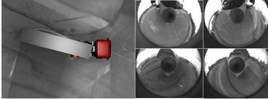
**Fig. 3.** Left: The bird's-eye view image. The kink angle between truck and trailer is  $-14^\circ$ . Right: raw images from the omnidirectional cameras.
