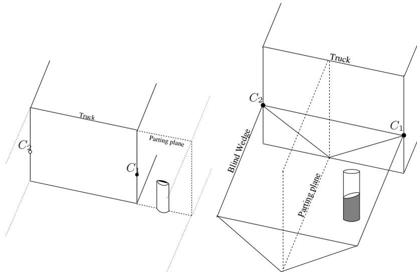
**Fig. 7.** Left: Splitting the space along the baseline of the cameras  $C_1$  and  $C_2$ . Camera  $C_1$  sees the black part of the cylinder and camera  $C_2$  sees the white part. There is no blind spot. Right: Splitting plane along the line of lateral symmetry of the truck. Everything that is within the blind wedge is not seen in the compound image. Thus, the empty part of the cylinder is not seen on the display (See also Figure 6).
