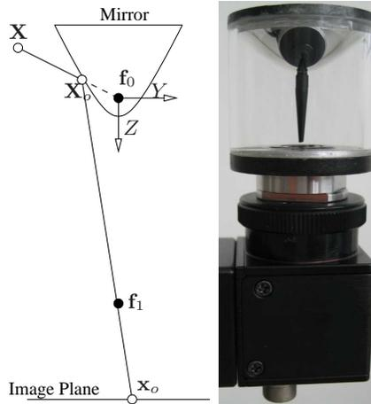
**Fig. 2.** The figure shows the omnidirectional projection. The point  $\mathbf{X}$  is given in the coordinate system defined by the focal point  $\mathbf{f}_0$  within the mirror. The z-axis points towards the image plane.  $\mathbf{f}_1$  is the second focal point with coordinates  $(0, 0, 2c)^T$ . Right: Omnidirectional camera consisting of a hyperbolic mirror with a standard pinhole camera. The black needle in the middle avoids reflections on the glass cylinder [10].
